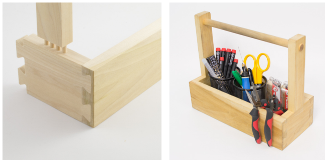
Figure 9. This poplar toolbox employs a variety of joints that would be difficult to create using current handheld and CNC tools.
